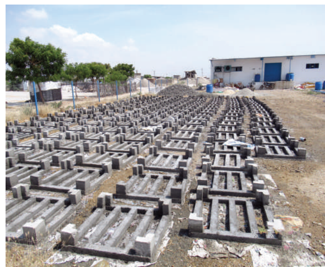
Construction of concrete frames
