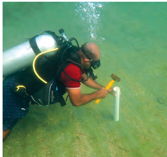
Fig. 19: Soil core sampling in mangrove, salt marsh and seagrass ecosystems
